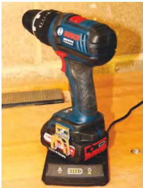
▲ As long as the tool or battery sits central to the charger, it will continue to charge
